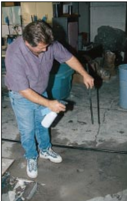
Figure 1. Form-release agent was sprayed on the rebar, covering 100% of the surface.
