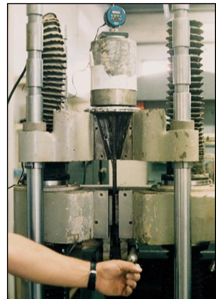
Figure 4. With the test specimen placed on a spherical bearing block on top of the testing machine, a tensile load was applied with serrated grips. An electronic digital indicator measured slip at the free end of the rebar.
