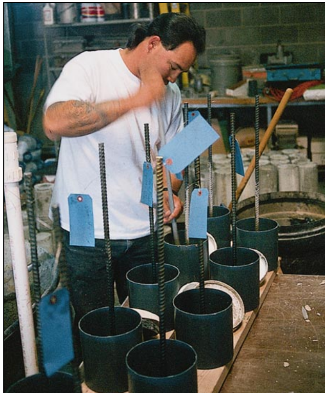
Figure 3. Pull-out specimens were cast in 6-inch-diameter, 6-inch-tall cylinder molds with a #4 rebar at least 24 inches long inserted at the center.
